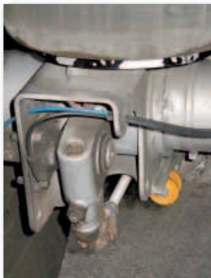
Stroke indicators (the yellow device) alert drivers to the need for brake adjustment.
