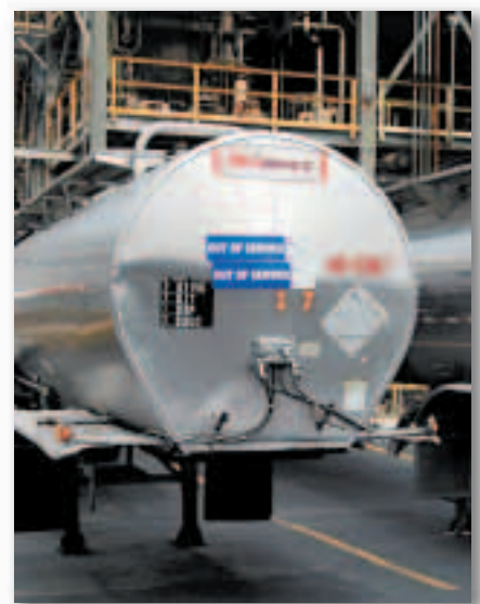
As part of the safety program, trailers that are out of service are clearly marked by an adhesive label that can't be easily removed.
