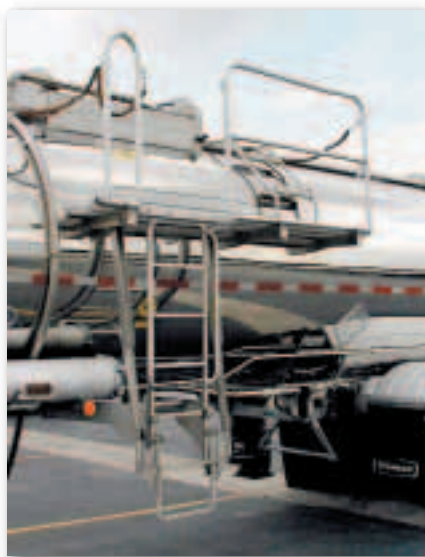
Trimac has been installing fold-down fall-protection railings on its tank trailers since 1992. Lowering the bottom rung of the ladder raises the railing.
