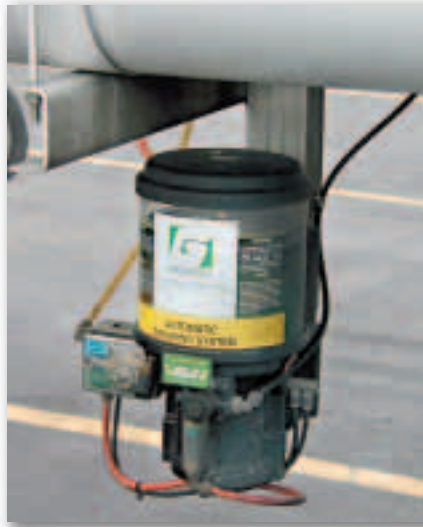
Groenveld's automatic lube system has extended preventive maintenance intervals for tractors and trailers. Trimac also hopes to increase tire life with the Meritor Tire Inflation System by PSI.
