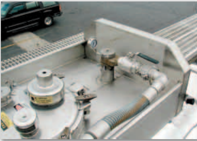
Tank hardware on chemical trailers includes Girard vapor recovery valves and pressure-relief vents.
